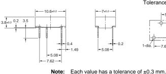
**PCB Mounting Holes** (Bottom View) Tolerance: ±0.1 mm
